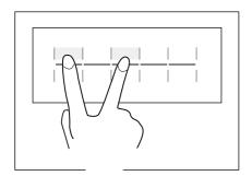
4. Press ▷|| to start the appliance, initially"---" is displayed, and then "\*\*\*" (such as "126")is displayed to indicate the real time drum speed. When the number reaches a certain value (stop changing),it means the washing machine is successfully calibrated.
