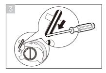
3.Pull down the emergency door pull cord (refer to direction of the arrow in the picture). If unlocked successfully, you will find the door lock icon will go out.
